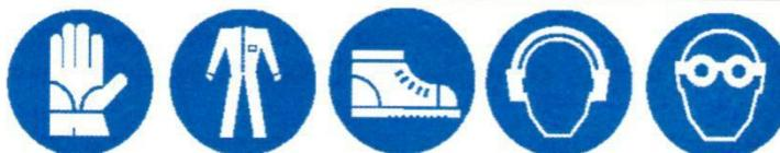
**The operator, during the period of using, maintenance, repairing, moving or storage of the machine, must wear accident-prevention shoes, overalls, safety gloves and if necessary anti-noise ear guards.**
